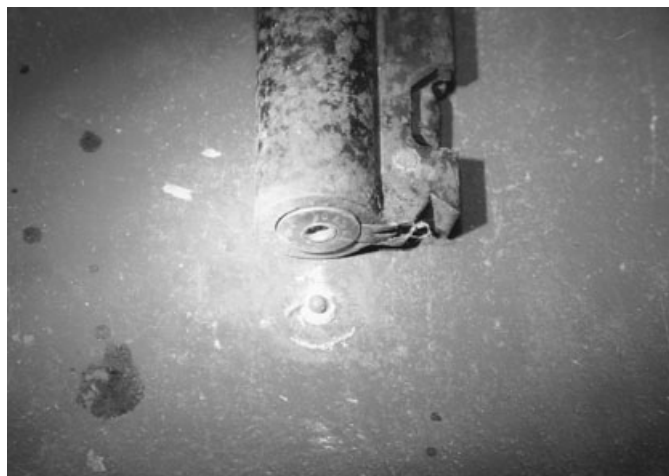
FIG. 4—Photograph of shotgun with shell casing as well as BB placed in indentation on the basement floor. The outline of the back of the shell casing is seen on the basement floor.
