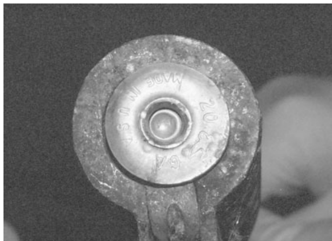
FIG. 3—Photograph of breech end of the shotgun barrel with spent shell casing. Note the multiple BB-sized indentations on the casing including the primer.
